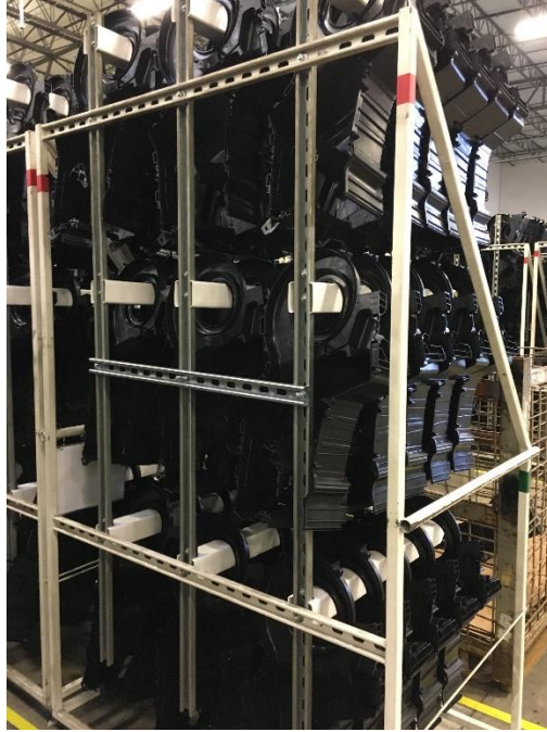
Figure V-2. Rear Steel Unistrut Stiffener
