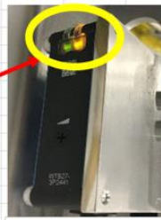
GREEN & YELLOW light= PART IN SLIDE, BREAKS SENSOR LINE
